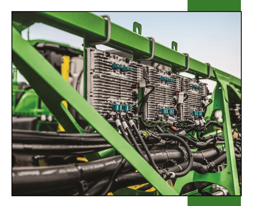
The system uses 36 cameras mounted on a 120 ft boom that look for any green plant material and then activate the appropriate nozzle to hit that target. This is all taking place at 12 mph, so the volume and speed of the computing power is truly impressive.
