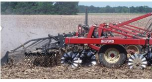
(On the left is a "seedbed conditioner" from McFarlane Manufacturing – arguably the builder of the first vertical tillage machine – on the right is a Salford 1100, featuring the contoured coulters, harrows and baskets that are commonly associated with vertical tillage units today)
